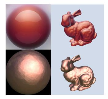
Figure 5. MatCap technique applied to a mesh
